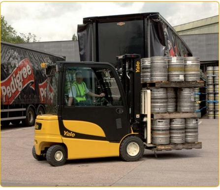
The Yale VL features a state-of-the-art extended steer-axle that has increased articulation of the steer wheels, allowing it to turn in smaller spaces than a conventional 4- wheel steer-axle.
