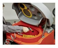
Easy-to-clean recovery tank: The recovery tank has a large opening to provide easy access. Particularly practical in combination with the spray nozzle (optional).
