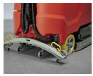
Daily maintenance and machine-cleaning made easy: The squeegee folds up manually.
