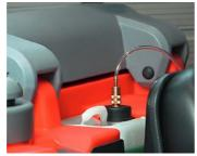
Adding the optimal amount of cleaning detergents in relation to the amount of water supplied in the cleaning process. The onboard dosing system is fully integrated into the machine design.
